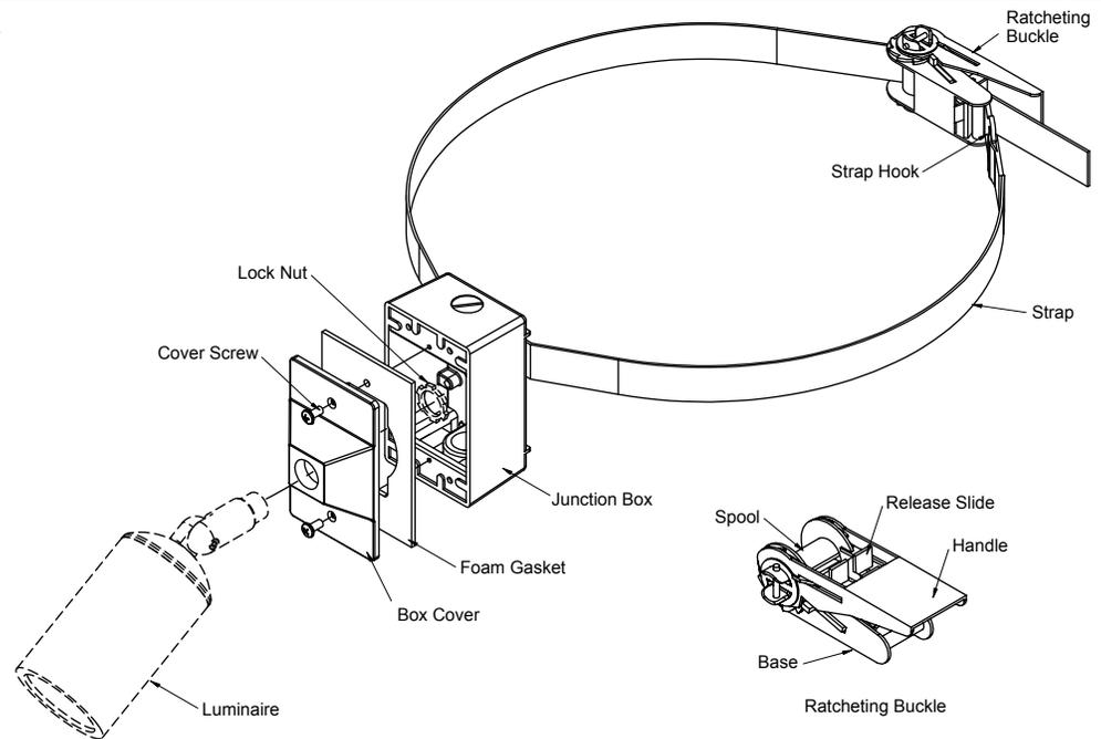
6. Tuck all wiring and connectors into the Junction Box
