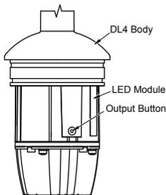
9. Install Cap on fixture by pushing and twisting slowly. If O-Ring is excessively dry, use a small amount of Krytox lubricant.
